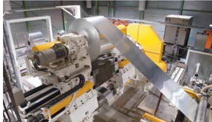
Unwinding and joining process ensures consistent 24/7 operation
