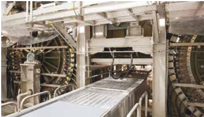
Electro-graining, the second stage, roughens the surface of the aluminium to improve water receptivity
