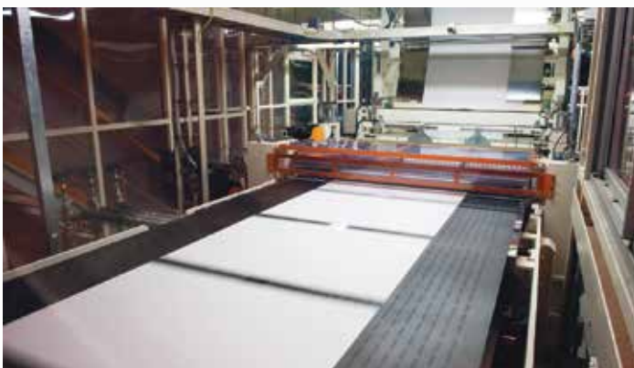
Interleaf paper is placed on top of the coated aluminium web just prior to cutting, protecting the plates before being packed
