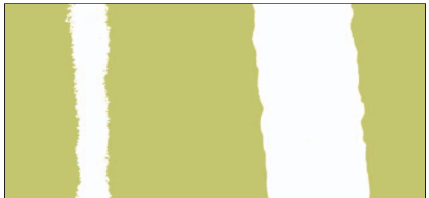
Illustration 1. Note the 1/2” (12.7 mm) equivalent FanBlast Nozzle with its wide pattern next to a conventional double venturi nozzle pattern. The FanBlast nozzle pattern width is 2.2” (5.6 cm) versus 5/8” (1.6 cm) average for the double venturi nozzle.
