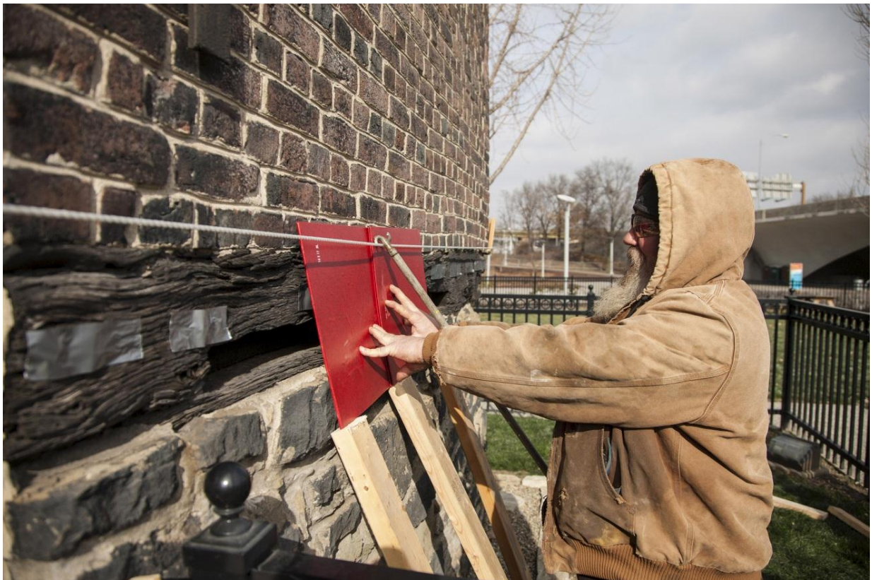
Phil Martin, Radiographer, is setting up the imaging plates for the next exposure during the radiographic inspection of the gun loops at the Fort Pitt Block House
