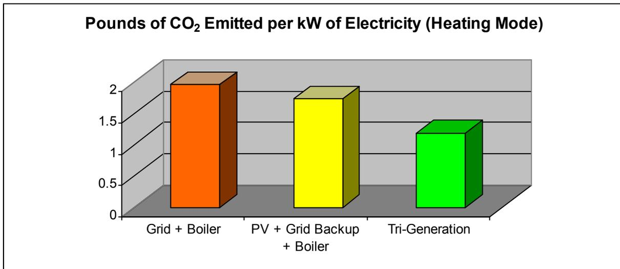
Even if the heat is not used, the solar PV system will emit 1.05 pounds per kW-hr while a reciprocating engine generator will emit 0.95 pounds per kW-hr. In New Jersey, the natural gas generator will emit less CO<sub>2</sub> than PV with grid backup even if the heat is not captured at all.
