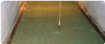
Post-test endurance results concluded that unvegetated GreenArmor 7020 exhibited a critical shear stress of 5.8 lb/ft 2 .
