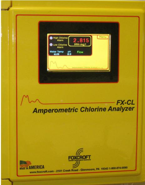
The Foxcroft FX-CL-D amperometric reagentless chlorine dioxide analyzer is available for continuous online measurements in clean filtered drinking water as well as for CIP (clean in place) processes or chlorine dioxide production. It operates without costly reagents and their associated maintenance.
