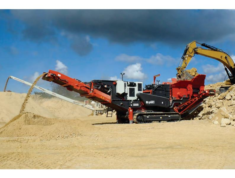
The QI441 is a heavy duty, tracked, self propelled impact crusher which features the unique Sandvik CI421 PriSec impact chamber, offering customers unparalleled flexibility through the ability to work in both primary and secondary applications.
