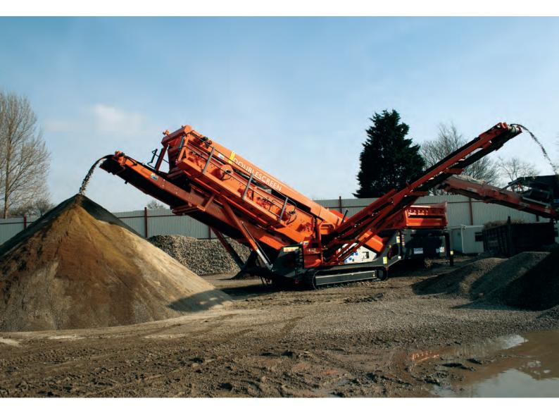
Building upon the highly advanced features of the QA440 and original QA450, the QA451 represents the second generation product with numerous product refinements, whilst retaining the triple deck screen box that enables it to produce up to four different product types plus one oversize.
