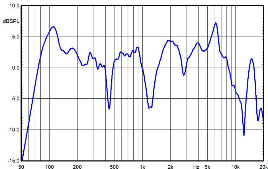
*Typical response of a woofer/tweeter combination in an inexpensive wireless speaker, with only a single capacitor used as the crossover circuit for the woofer and tweeter. Ideally, this line would appear flat.*
