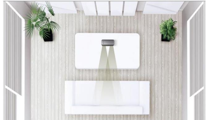
*Electrostatic drivers emit sound freely forward and backward, so they have a more spacious, natural sound. Conventional full-range drivers emit sound only forward; sound coming from the rear of the driver resonates inside the enclosure.*
