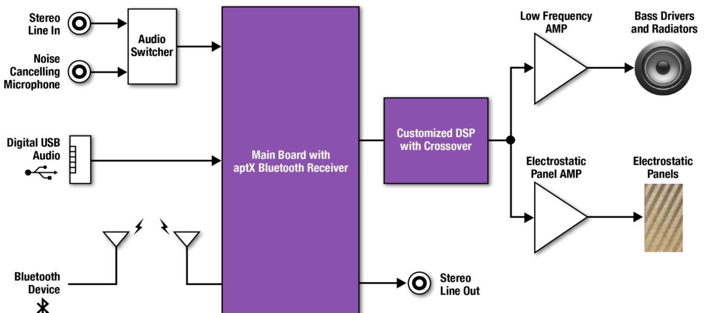
*Because a separate amplifier channel is devoted to each driver in the treVolo, all of the crossover and EQ functions can be implemented in DSP, instead of using passive components.*
