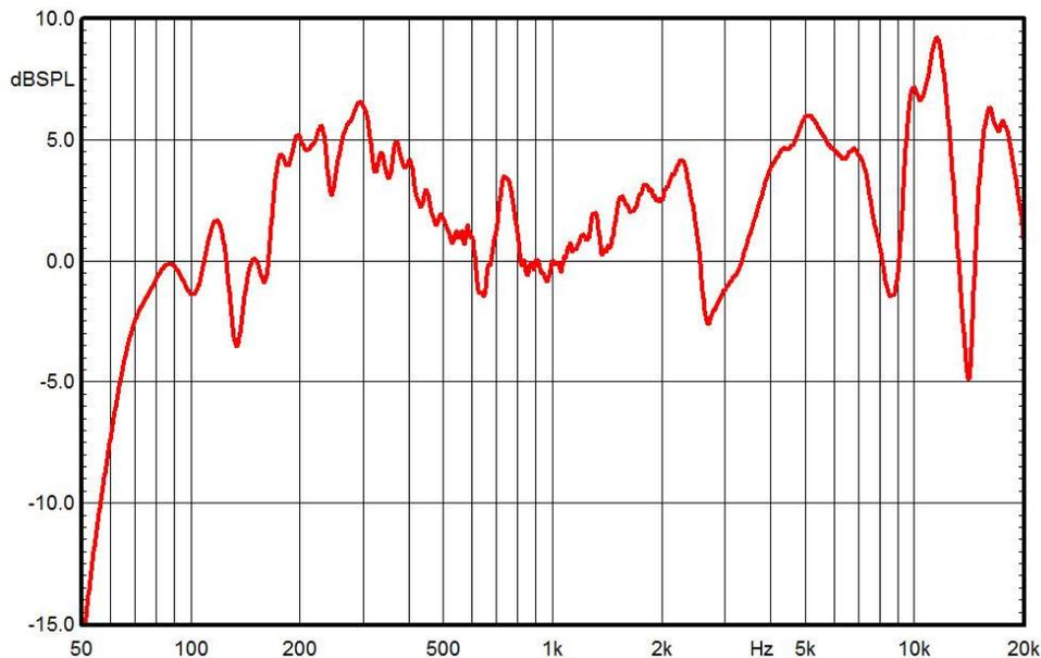
*Typical response of a full-range cone-type driver. The flatter the red line is, the better. Large peaks and dips in the response make the sound unnatural.*
