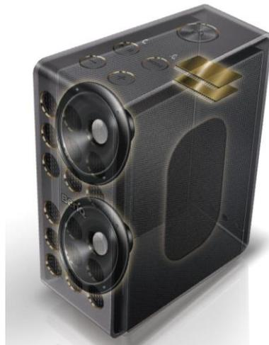
*The treVolo uses dual 2.5” woofers and large passive radiators to generate crisp, accurate bass. These drivers operate on a separate amplification system than the electrostatic panels and are controlled via the DSP for smooth transitions from low to high frequencies.*
