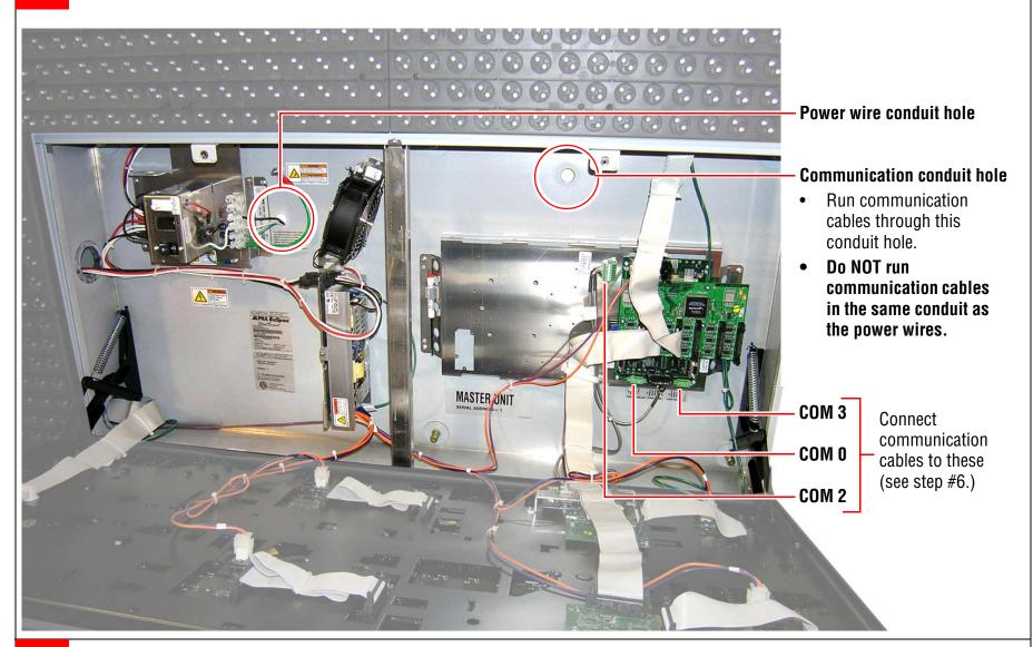
Wire the communication cables to the MASTER and SLAVE signs as shown below:
