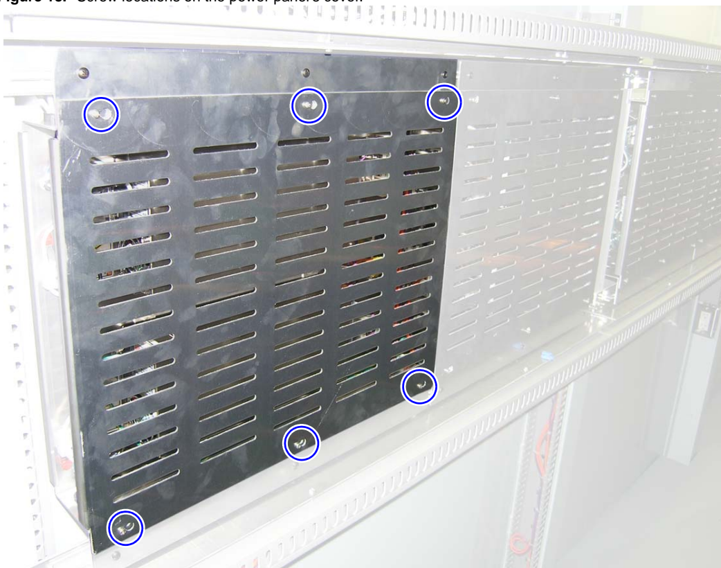
Figure 18. Screw locations on the power panel's cover.
