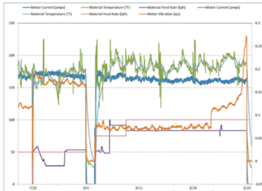
Figure 1. A deluge of data: Trend data as shown in the image above is typical in production environments. Although not obvious to the naked eye, staff are often required to interpolate the trends of numerous asset attributes and to discern subtle changes in an asset's condition.
