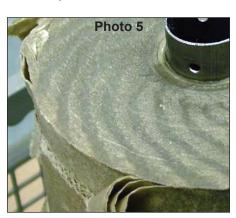
In rolled axial flow elements (see photo 5) the fluid enters the element through the end and must turn to pass through the media. The effective area through which the fluid must pass in a rolled media element is exponentially smaller than the flow area of a pleated, radial flow element (see photo 4).
