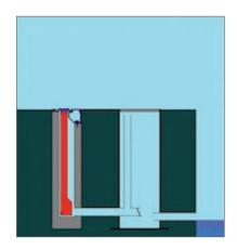
In storage position, all operational parts of the barrier are concealed in an underground storage basin. The basin in covered with a connected lid and is flush to adjacent ground.
