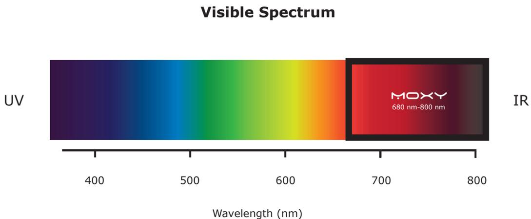
Near-Infrared light works well for this type of measurement because it can travel for long distances through skin, fat, and muscle without being completely absorbed. The light is scattered through the tissue rather than traveling in a straight line, which makes quantifiable measurements a bit challenging but still possible.
