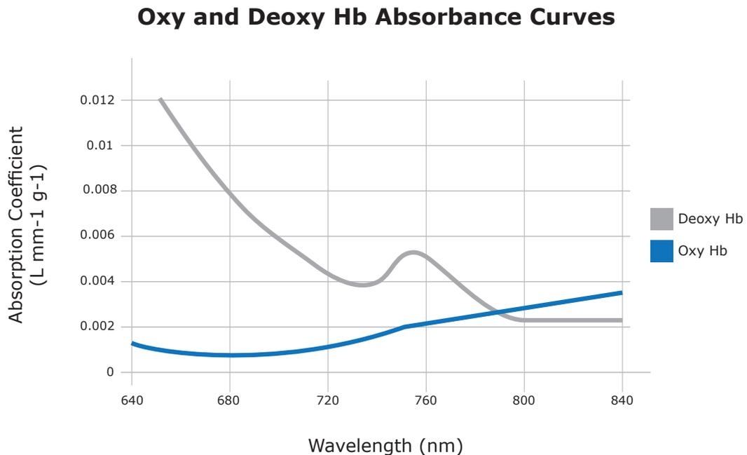
In order to use NIRS to take quantifiable measurements in human tissue, a model is required to calibrate the measurement system. Some devices use a physical model like a tissue phantom or actual human measurements. Moxy uses a theoretical model because it allows the accommodation of a much wider range of physiologic variables, and the only cost is working out some challenging mathematics. Moxy uses a four-layered tissue model consisting of epidermis, dermis, fat, and muscle.
