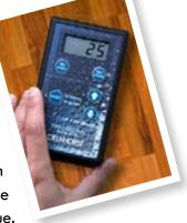
Construction crews and contractors employ moisture meters to verify the %MC of flooring, structural lumber, and the RH of concrete to ensure that the construction job can proceed without the risk of buckling, warping, or other problems.
