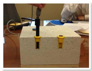
To that end, ASTM F2170-11 recommends the use of in situ probes to obtain accurate relative humidity measurements. This is a big improvement over the calcium chloride testing which is less reliable in that calcium chloride testing only indicates moisture in the top 1/8", and are prone to false positives.
