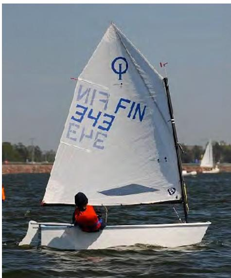
*Fig. Small wrinkles perpendicular to the sprit are completely ok!*
