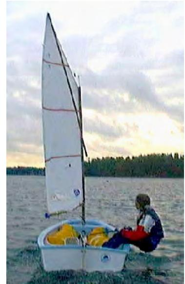
Basically, the sail is sheeted so that the boom is above the leeward corner. The telltale at the back end of the top batten should fly at least 50% of the time. If it is most of the time stalled behind the sail, you need to twist the sail more open by easing the sheet, sprit or vang. In stronger winds, when getting over-powered, the telltale should, of course, fly all the time.
