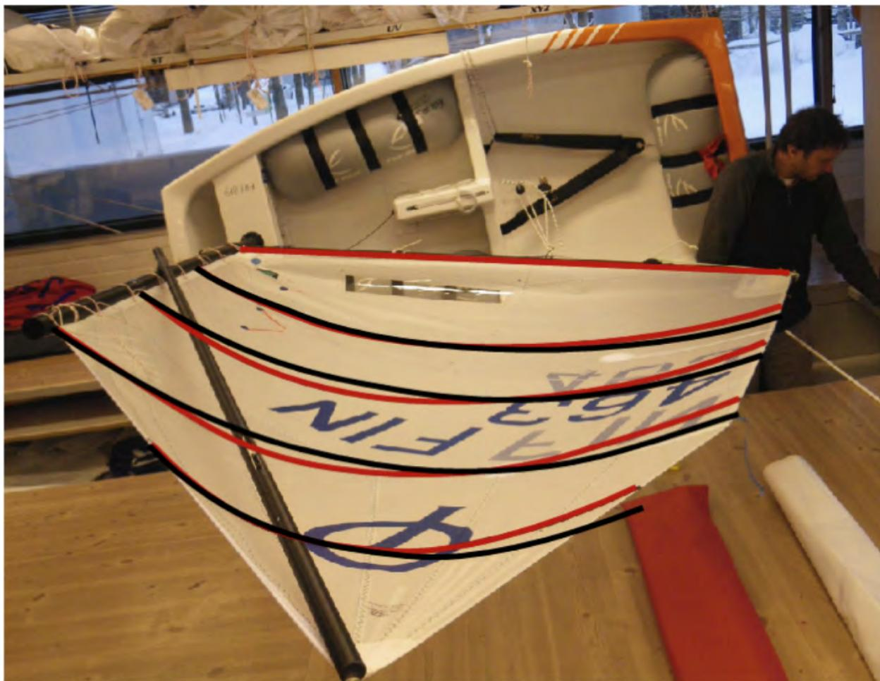
*Fig. The effects of the sprit tension. The red curves are showing a tighter sprit, and black curves a looser sprit.*
