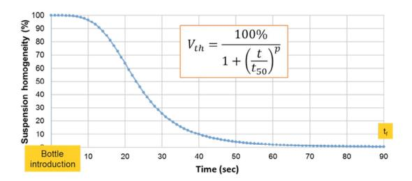
On a typical example, the changes in the concentration would affect the curves modifying both the exponent p and the  $t_{50}$ . The biomagnetic separation is a cooperative behavior where the beads interact between them through magnetic dipolar interaction (overcoming the thermal agitation). The higher the concentration the nearer the magnetic beads would
