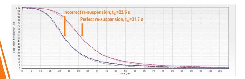
By recording the transmitted light across the vessel, we can monitor the transparency changes during the separation process, showing the describer sigmoidallike behavior. As shown in the figure (real case), using the same suspension in the same SEPMAG® Q1L, the time is reduced by almost a 30% when beads have become aggregated due to a bad storage protocol.
