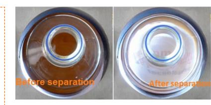
To address this issue, Advanced Biomagnetic Separation systems monitor transparency changes during the whole separation process. The resultant curves give a quantitative value of the transparency at the end of the process, and also show how it changes since the vessel is introduced in the magnetic separation rack. Properly recorded, these graphs would allow comparing the successive batches, and generating reference curves.
