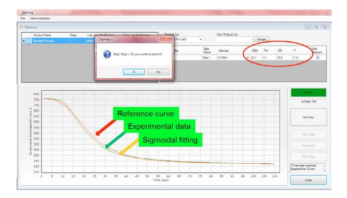
We can take advantage of this behavior to stablish quality control protocols that can indicate re-suspension problems during the biomagnetic separation steps. A reference curve can be generated for each step and the experimental curve obtained during the process. Any significant deviation from it would be
