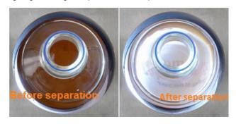
This method can be used with different wave lengths, using spectrophotometry if necessary. It is likely to improve accuracy, however, the system needs to be tailored to the bead/particle and suspension. The correct wavelength for a 50 nm magnetic particle is not the same as that for a 1 micron magnetic bead. A simpler approach, measuring white light transmittance, has proven effective for a wide range of diameters and buffers.
