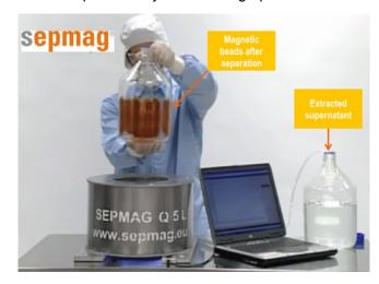
The only way to overcome these significant material losses from standard biomagnetic separators is to switch to more modern systems that generate homogenous force conditions regardless of the distance from the beads to the magnet.
