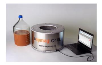
A well-defined magnetic force is a force that is high enough for the beads to be magnetically saturated, but low enough that irreversibly aggregated beads do not form. The force must also be high enough to retain the beads during supernatant removal. With the optimal magnetic forces known for various volumes, the only parameter that needs to be determined in the new volume is the correct time of separation. The separation time for larger systems can be estimated as:
