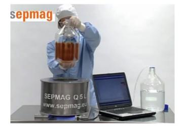
One option is to increase the size and weight of the magnetic separation device. This helps you gain increased magnetic force over the farthest beads, but doing so will also have a deleterious effect on the beads already in the retention area. When these beads are exposed to high forces over long periods of time, irreversible aggregation becomes a very se-
