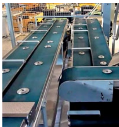
Optimum arrangement: The out-of-strip method facilitates the correctly oriented transfer of parts after the fineblanking process.
