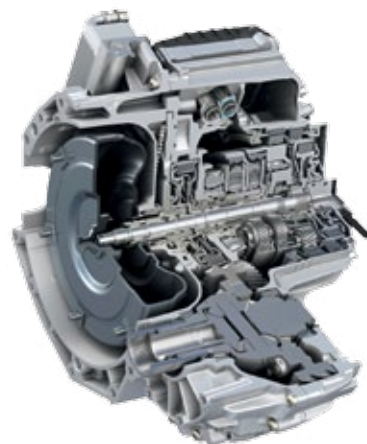
Advanced 9-speed FWD transmission using precision formed Feintool parts
