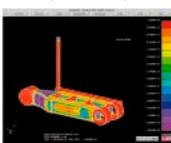
**CADDS5**<sup>™</sup>, from Computervision , is used for three-dimensional models of the part before patterns are produced.
