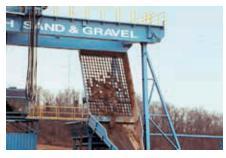
Hydraulically actuated dump grizzly for oversize material and clay removal
