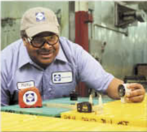
Delivering the best screen for your application is our only goal at TEMA Isenmann. We check aperture, base height and material on every screen. Using durometers, our quality control technicians also ensure proper screen hardness before your panels leave the plant.
