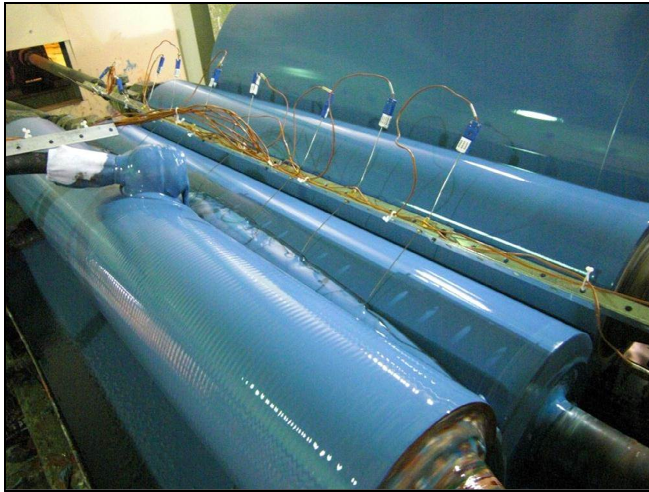
Figure 14: Measuring Temperatures in a Roll Coating System
