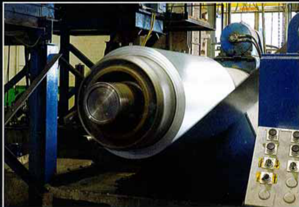
Metal strip moves onto the recoiler at Centria's Ambridge, PA facility. p. 12
