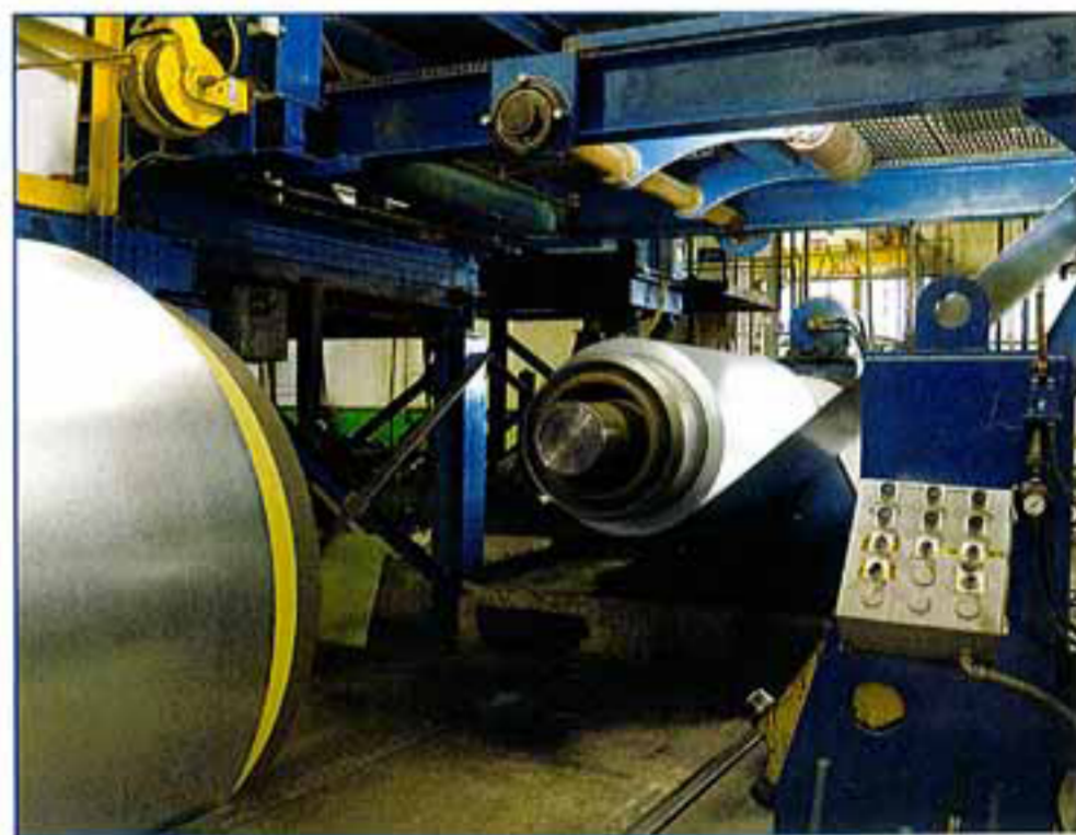
A metal strip moves onto the recoiler prior to the coil being prepared for packaging.
