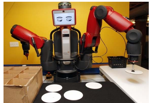
Rethink Robotics: Flagship product, Baxter, designed to work alongside people: Baxter is the flagship product built by the company and is billed as America’s first adaptive manufacturing robot.
