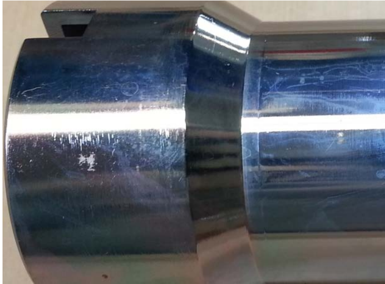
Figure 2 - Electropolish 'frosting' post coating without the aid of a white LED
