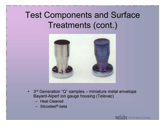
There was also a comparison of Heat Cleaned vs. Silcosteel-UHV coated gauge housings on an lon pump system. Thanks to Televac for supplying the housings.
