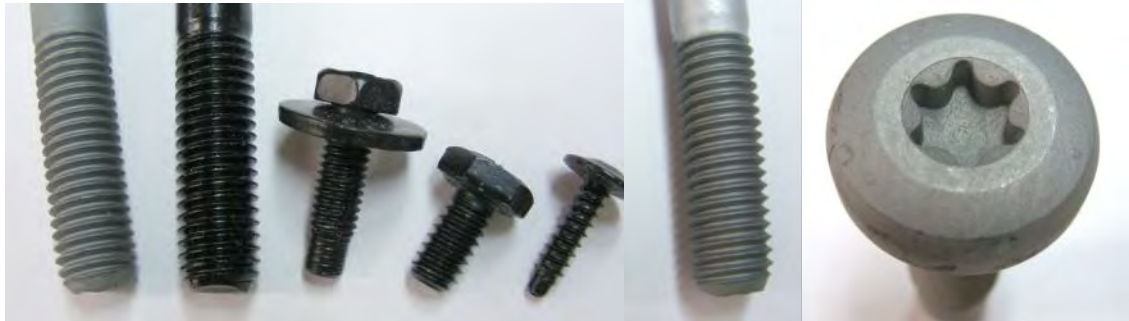
FIGURE 31 – Thread and Recess Fill - Left to Right, zinc rich M10, (zinc rich plus E-coat M10, M6, M6, M4), Zinc rich plus Aluminum rich topcoat (2 coats) M10, Zinc rich M10 recessed head.
