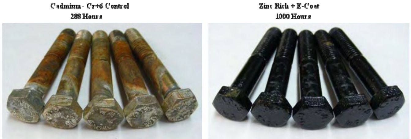
FIGURE 28 – ASTM G85 SO 2 Salt Spray
