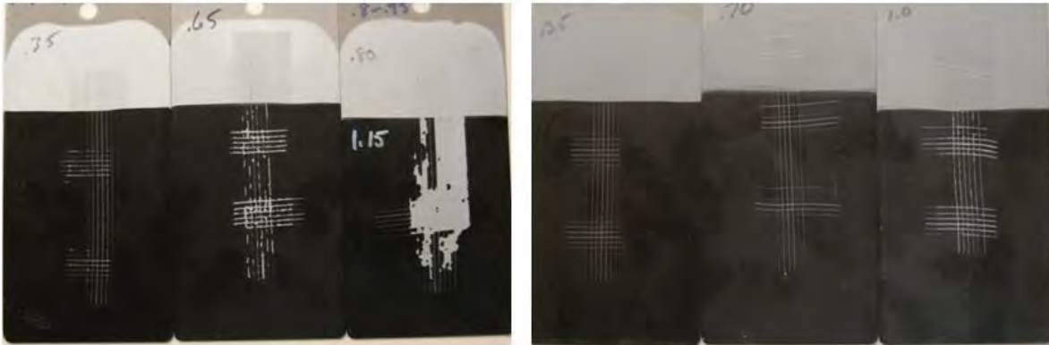
FIGURE 29 – Adhesion / Cohesion versus Primer Film Thickness
