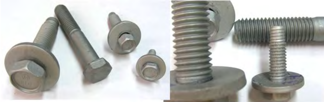
FIGURE 19 – Aluminum Rich Topcoat Appearance and Thread Performance
