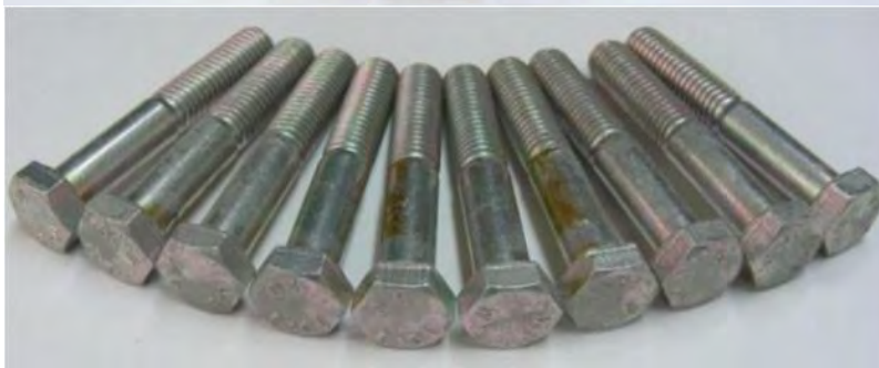
FIGURE 23 – Salt Spray Corrosion Results
