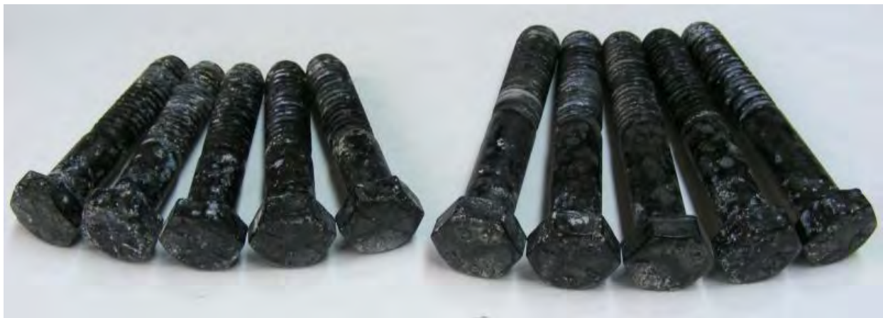
FIGURE 27 – GM9540P – 100 Cycles – No Red Corrosion
