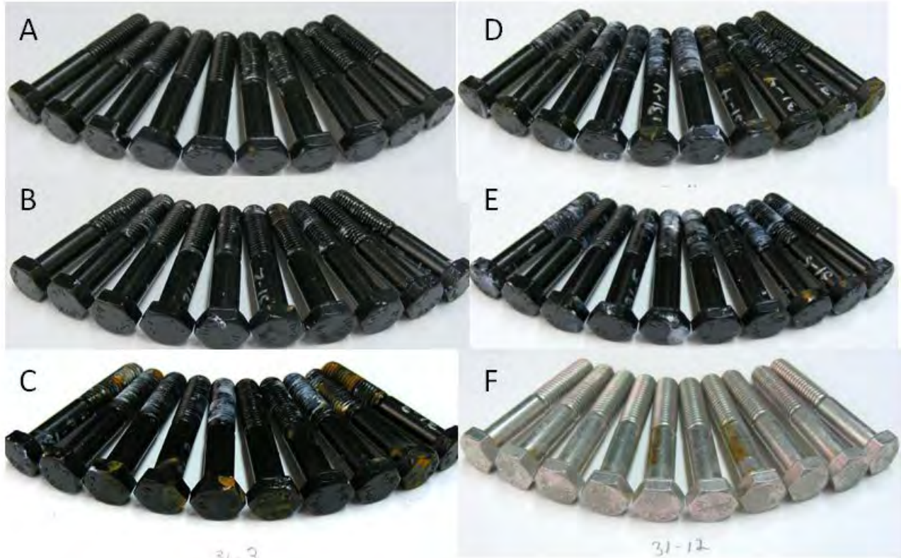
FIGURE 4 – Test Bolts – 1000 Hours B117 Salt Spray – Pretreatment Variations
