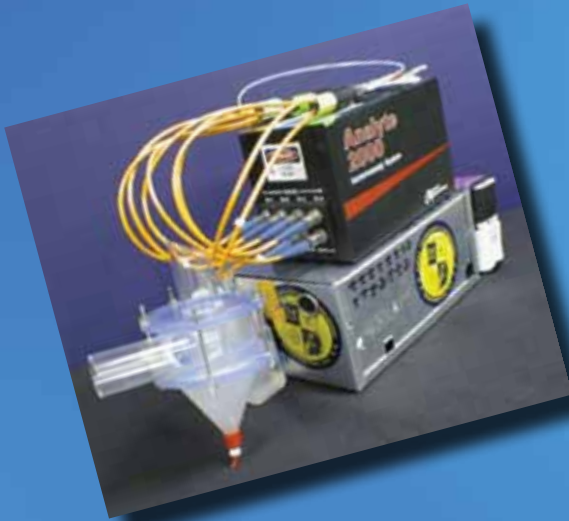
Analyte 2000 Fiber Optic Biosensor (1998) — As payload on the Swallow UAV, NRL's biosensor provided one of the first demonstrations of the identification of aerosolized bacteria by a sensor flown on a remotely piloted plane, with data transmitted to a ground station.
