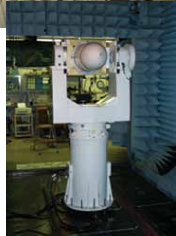
Radio Frequency Countermeasures anechoic chamber for EW testing.
