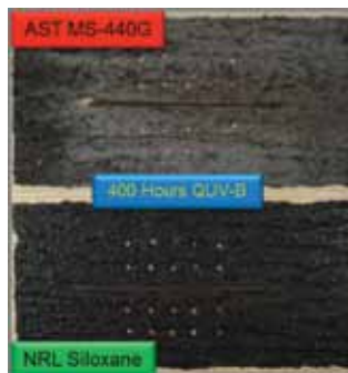
Comparison of a legacy nonskid coating to an NRL-developed organosiloxane nonskid coating. Left: Five-month service comparing legacy nonskid to NRL organosiloxane applied to the USS Ponce LPD 15. The NRL system holds its deck gray color while the legacy nonskid systems degrade to an ocean gray from solar radiation. Right: Two 6-in. x 12-in. x 1/4-in. steel plates. The lower plate is coated with the NRL organosiloxane, while the upper plate is coated with the legacy nonskid. 400 hours of accelerated UV testing show the improved color stability of the NRL system over the legacy system.
