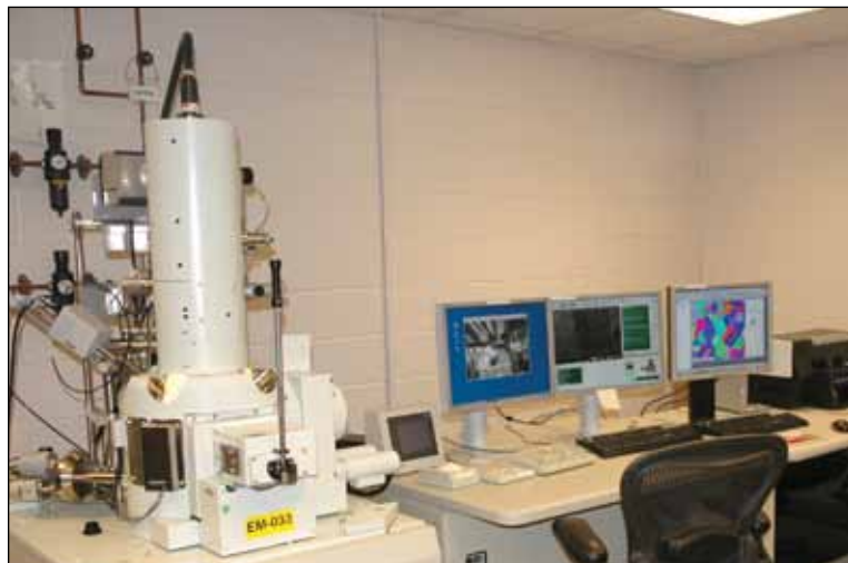
The JEOL JSM 7001FLV Variable Pressure Field Emission Scanning Electron Microscope, outfitted with EDS and EBSD capabilities.
