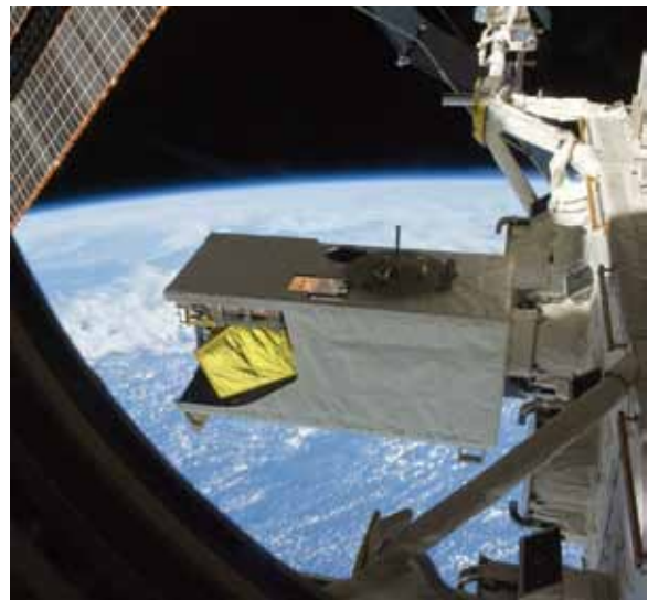
The Hyperspectral Imager for Coastal Ocean (HICO) and Remote Atmospheric and Ionospheric Detection System (RAIDS) Experiment Payload (HREP) installed on the Japanese Experiment Module Exposed Facility on the ISS. In this view from the Japanese Experiment Module window, the gold-blanketed RAIDS scan head is tipped down to make extreme ultraviolet measurements of the Earth's daytime ionosphere below the ISS. (Photo credit: NASA)
