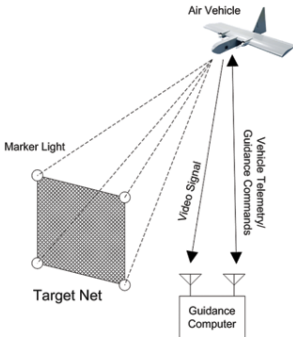
FIGURE 1 Vision-based automatic recovery system diagram.
