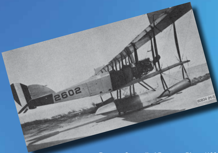
Remote-Controlled Pontoon Plane (1924) — NRL developed the control system for the first U.S. flight of a radio-controlled pilotless aircraft. Remotely controlled from the ground, the N-9 float plane took off from the Potomac River, followed a triangular course, executed glides and climbs, and landed on the river.
