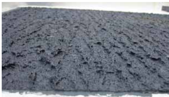
FIGURE 1 Close-up view of NRL's siloxane nonskid coating (rolled version).
