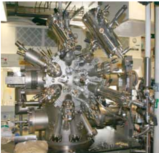
Molecular beam epitaxy (MBE) system dedicated to quantum confined GaSb/InAs/AlSb structures for mid-wave infrared laser development.
