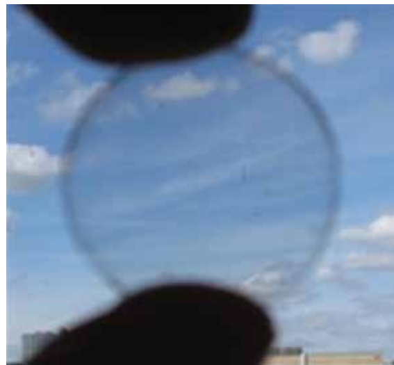
FIGURE 2 A polished 1-in.-diameter transparent 10% \text{Yb}^{3+} doped \text{Lu}_2\text{O}_3 ceramic sample.
