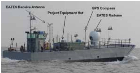
EATES — Electronic Attack Technique Evaluation System, a stand-alone portable EA testing system.
