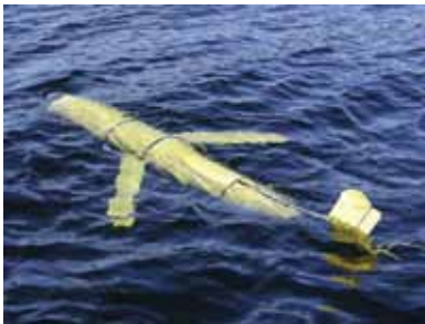
Slocum gliders, autonomous underwater vehicles, are equipped with temperature/salinity/pressure sensors and with real-time satellite connection to the Iridium network.
