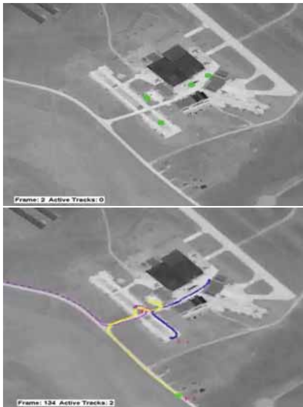
FIGURE 9 Top: Track initiations, indicated by green markers. Bottom: Track generation for three vehicles, T:1, T:2, and T:3.
