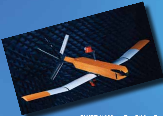
FLYRT (1993) — The FLYing Radar Target RF-distraction decoy flew at ship-like speeds following launch from a shipboard chaff launcher. The fiber optic gyroscope provided highly accurate angle rate data.
