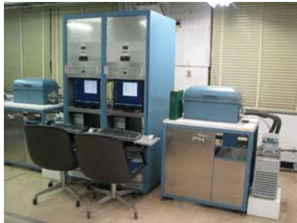
FIGURE 10 One of the closed vacuum chambers and equipment racks containing the data collection and monitoring systems.
