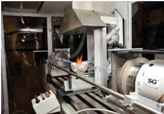
The Optical Fiber Preform Fabrication Facility includes computer control of the glass composition and standard fiber-optic dopants as well as rare earths, aluminum, and other components for specialty fibers.
