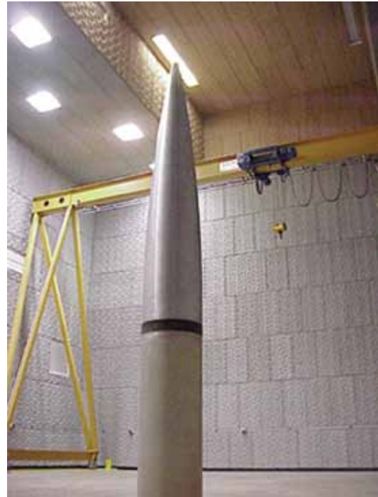
The Structural Acoustics In-Air Facility is instrumented with acoustic and vibration measurement systems for conducting ultra-high-precision, highly spatially sampled measurements on scaled submarine structures, satellite payload fairings, active and passive material systems for sound control, and new transducer and sensor systems.
