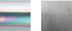
The different colors of the coating can be attributed to angstrom-level thickness variations across the surface. All SilcoTek coatings have a thickness of <math><1.5\mu\text{m}</math>. Certain coating processes (e.g. Silcolloy, SilcoGuard) result in a thicker layer and have a silver/matte gray appearance, while thinner coatings (e.g. SilcoNert) exhibit the "rainbow" colors.
