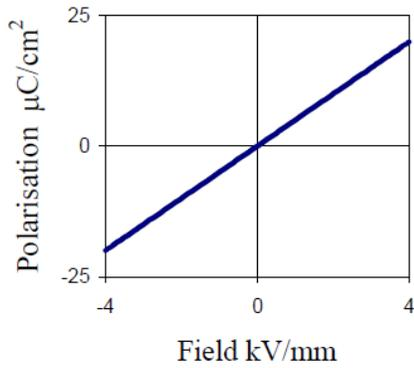
Figure 1a): Ideal linear capacitor response
