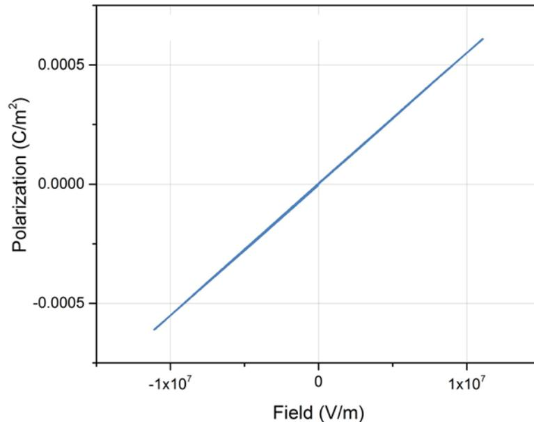
Figure 4): P-E response of the current Dursan coating
