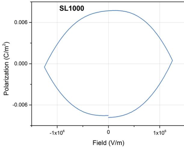
Figure 2a): P-E response of Silcolloy 1000 coating
