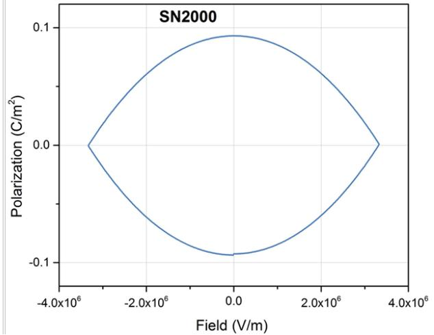
Figure 2b): P-E response of SilcoNert 2000 coating
