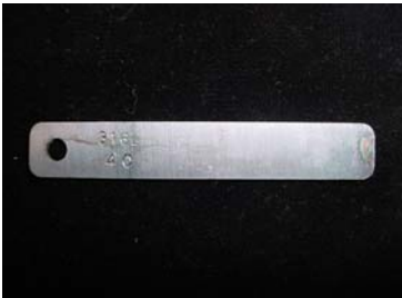
FIGURE 6 - Photograph of silicon treated 316L SS after 4000 hours salt spray exposure
