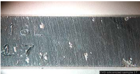
FIGURE 4 – Photograph of Silicon Treated 316L SS after 72 hour exposure to 6N ferric chloride
