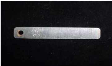
FIGURE 7 – Photograph of untreated 316L SS after 4000 hours salt spray exposure
