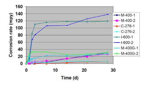
Studies have shown that the presence of oxygen in the HF vapor dramatically increased the corrosion rate of alloy 400. Alloy C-276 is also adversely by temperature and oxygen but not as adversely as alloy 400. Additional data from Haynes International Inc. also strongly supports the use of Ni-Cr-Mo alloys<sup>2</sup> like alloy C-276 for HF service in the presence of oxidizers for temperatures up 80°C.
