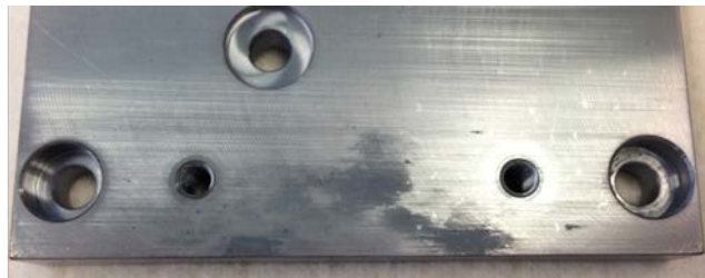
Figure 5. Organic contamination that cannot be removed by SilcoTek's cleaning process.
