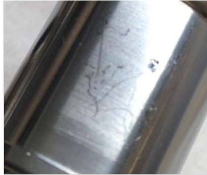
Figure 6. Scratches on incoming parts identified at SilcoTek's receipt inspection.
