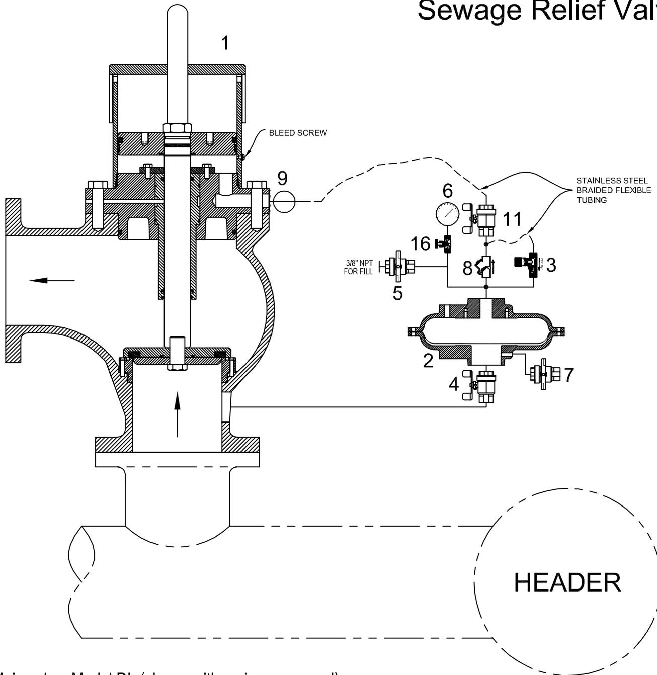
1. Main valve, Model DL (shown with springs removed).
