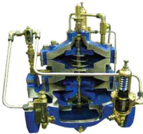
Should the primary pilot system and / or main valve fail to control the downstream pressure, the independent back-up pilot system will begin to operate. It controls the pressure above the diaphragm in the second operating chamber. The back-up pilot is set slightly higher than the primary pilot. The forces now operating in the top chamber assume control of the inner valve assembly and maintain pressure reducing control.
