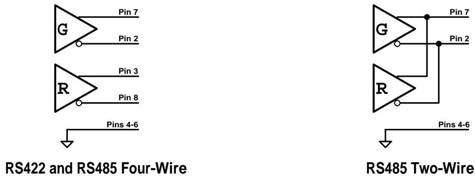
Figure 7 – P1: Isolated Serial Interface Pinout - RS422/485 Configuration
