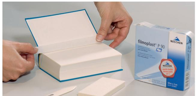
The tape has a pH of approximately 7.5 and is not buffered. Like the original, filmoplast® P 90 plus will not dry out or become brittle with age and is ready to use off the roll with no wetting required.
