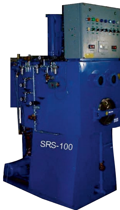
For printers, various distillation stages in this automatic system permit the reuse of solvent, instead of its usual disposal off site.
