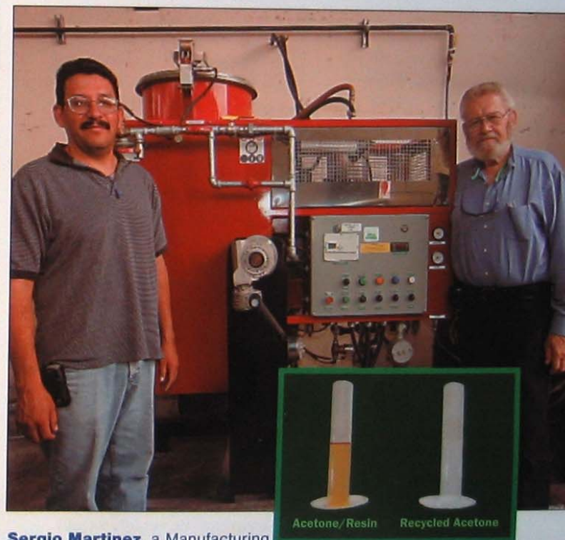
Sergio Martinez , a Manufacturing Engineer and Norm Dunavant , one of the original founders of SCI and a current consultant to the company, stand in front of the acetone recovery and disposal machines. Insert shows the before and after of the Acetone Recycling Process.
