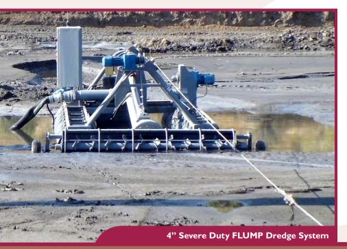
Meet the **FLUMP,** our remote-controlled dredging system for continuous removal of settled solids.
