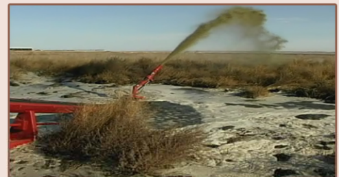
Nozzle adjusts to 74 degrees of vertical movement and 320 degrees of rotation
