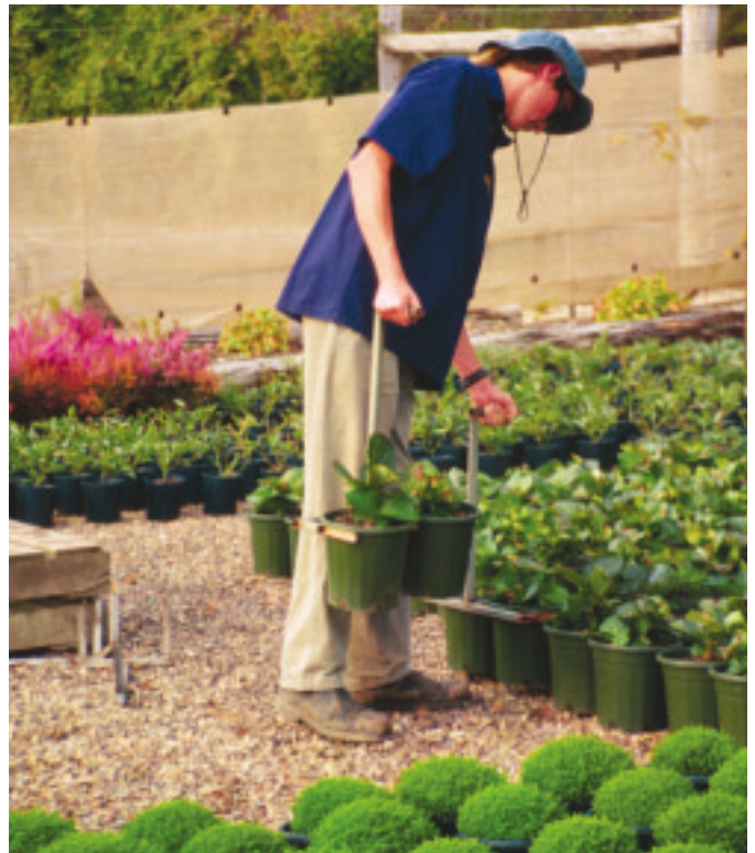
Back problems are common in our industry. Simple lifting devices can help. Bournda Plants, NSW.
