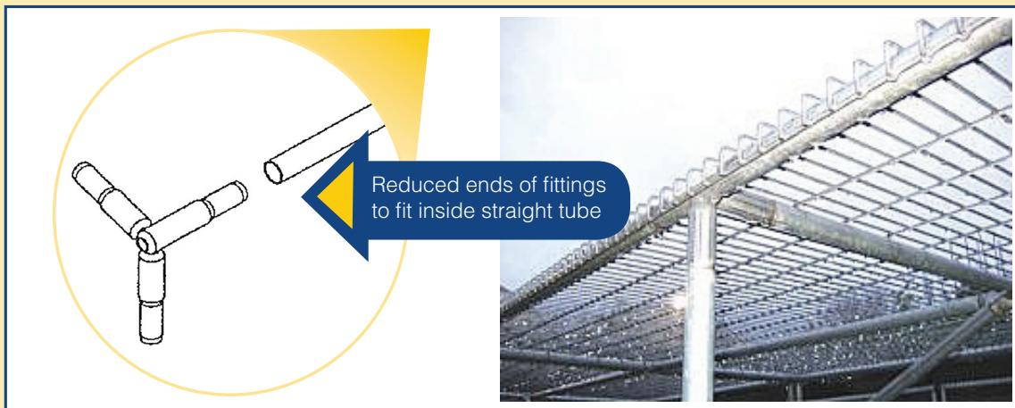
“Spring Benches” can be assembled in a few minutes without the need for any bolts, screws or other fasteners. The various tubes simply slide into the appropriate sockets to create a strong assembly. Even after twenty years the benches can be disassembled simply by pulling them apart, providing a smear of petroleum jelly has been applied inside the fittings before assembly.
