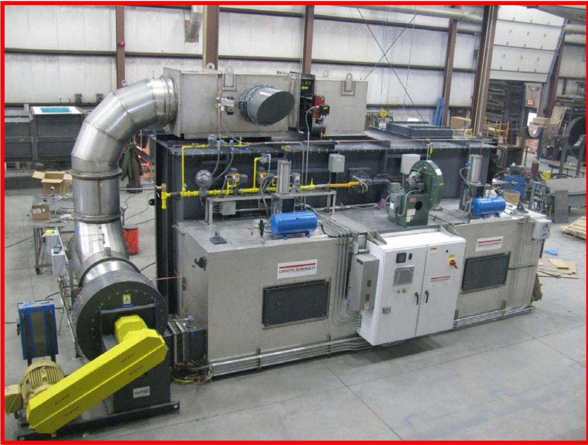
**Hot Air Recirculation** – mixes clean hot oxidizer exhaust with cold wet inlet gas to insure re-vaporization of condensing water vapor prior to entering the EvenFlow Manifolds.
