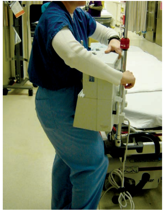
Figure 7.6. This heavy device has an awkward screw clamp, so this nurse is trying to support its weight with her leg while she gets the device fastened to the pole.
