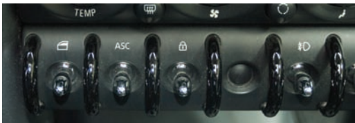
Figure 21.17. These switches in my MINI Cooper S look slick but don't show state very well because they return to the same position regardless of whether they are activated. There's a tiny LED at the end of the switch for traction control, but it's so invisible it might as well not be there.
