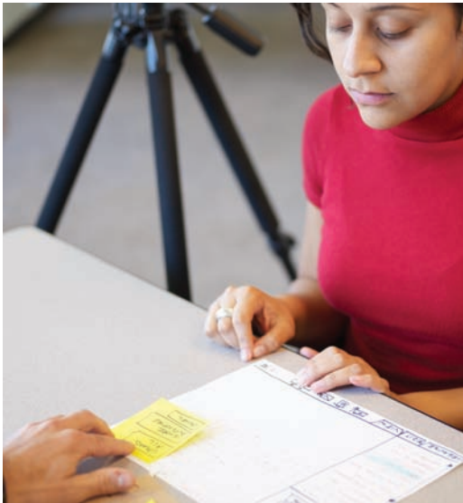
Figure 23.1. An inexpensive usability test using a paper prototype and basic camcorder.
