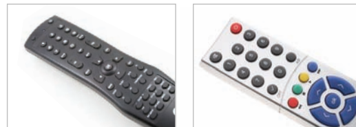
Figure 21.8. The remote control on the left does not have a clear visual hierarchy. The remote on the right at least highlights important functions with color, though the choice of green for a stop button is unfortunate.
