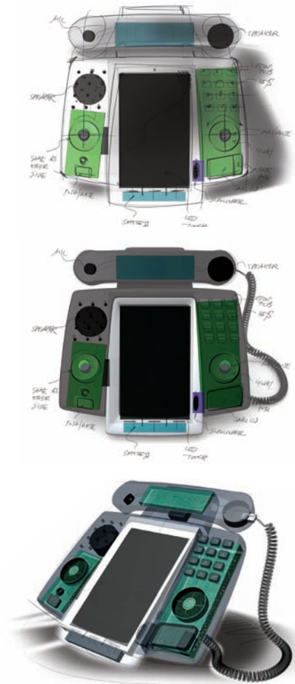
Figure 16.5. Industrial designers must consider internal components early on.
